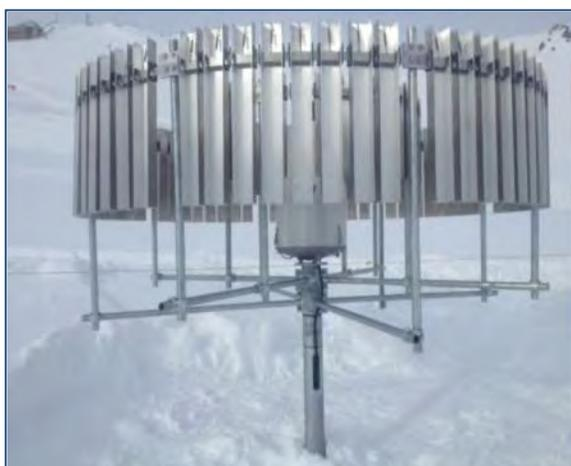
**Belfort Precipitation Gauge and Wind Shield attached to top of mounting pole in Davos, Switzerland**
