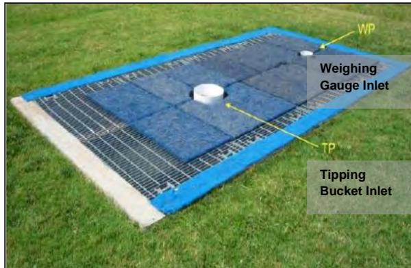
Pit Site for Precipitation Gauges can be subject to blowing snow and debris, C.E. Duchon et.al 2010, University of Oklahoma
